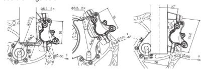
The specifications of the hubs for Y-2 disc brake system is the same as international standards, see drawings below:
